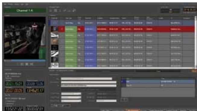
▲ Cuba HDP is a 24/7 channel-in-a-box playout system that combines video playout, on-air graphics, playlist and transfer management in a single server.
